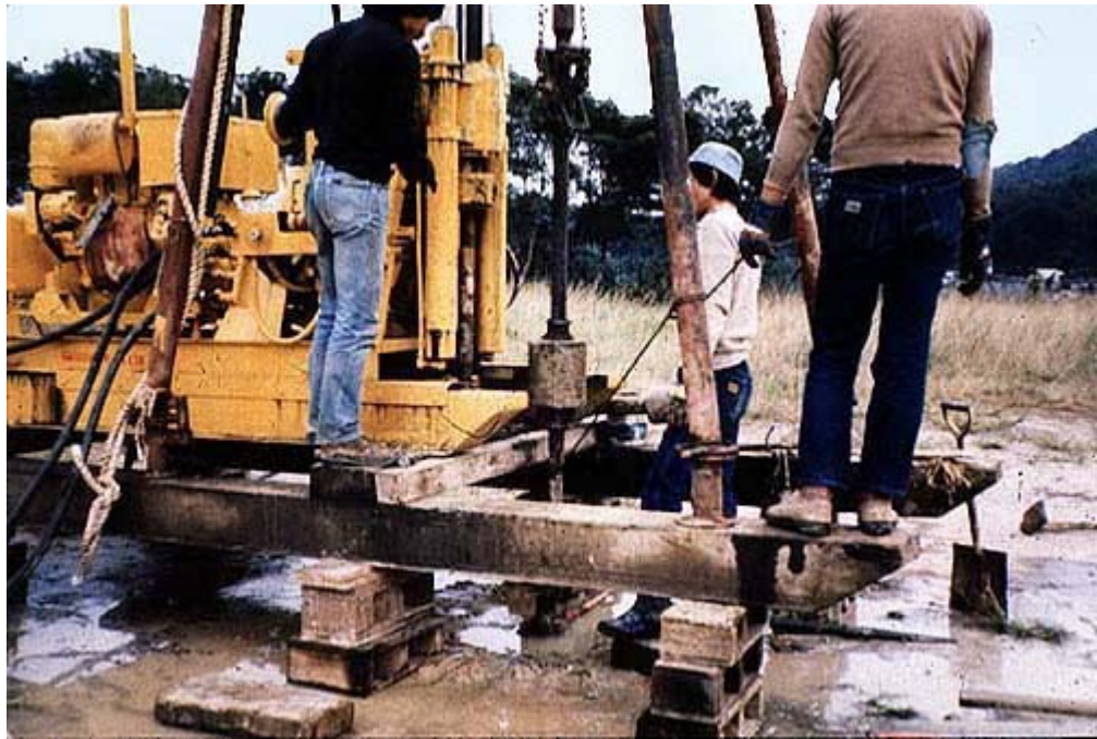
Standard Penetration Test (SPT)
