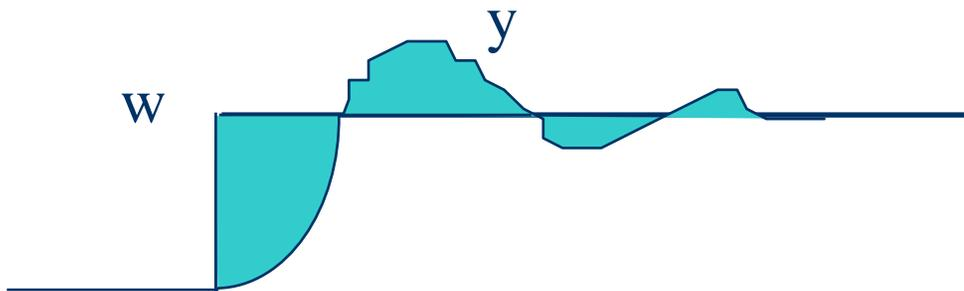
$$\min_{K_p, T_i, T_d} \int e(t)^2 dt \quad \text{MISE}$$
