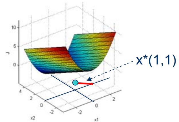
$$\left. \begin{array}{l} \min_{x_1, x_2} x_1^2 - x_2 \\ x_1 + x_2 = 2 \\ x_1^2 + x_2^2 \leq 4 \\ -x_1 + 1 \leq 0 \end{array} \right\}$$
