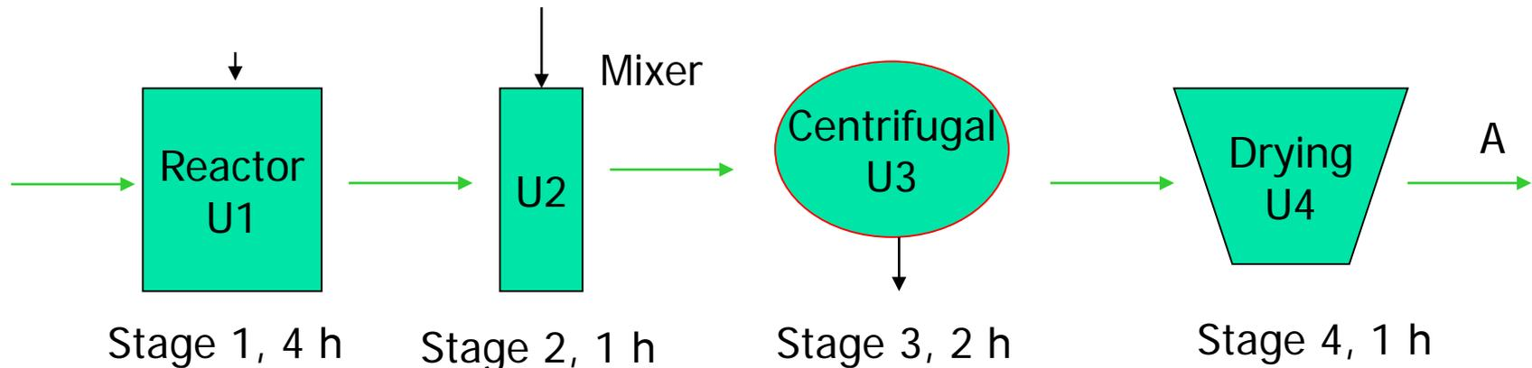
In the example, manufacturing of product A cover four successive stages (each one in a different batch unit, lasting the indicated times )
