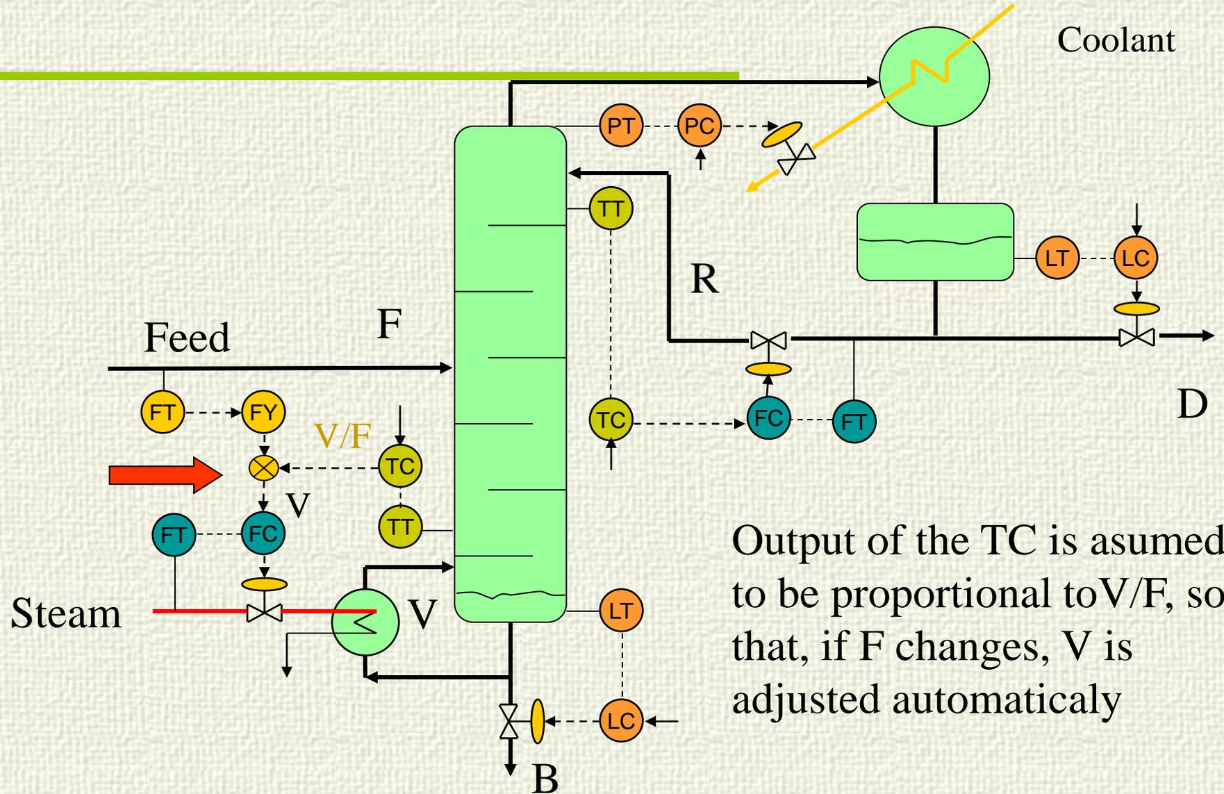
Output of the TC is assumed to be proportional to  $V/F$ , so that, if  $F$  changes,  $V$  is adjusted automatically
