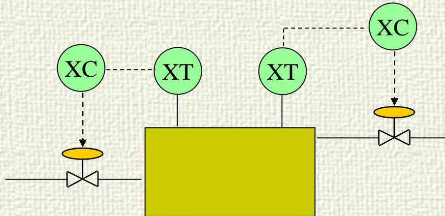
One variable should be controlled using only one controller
