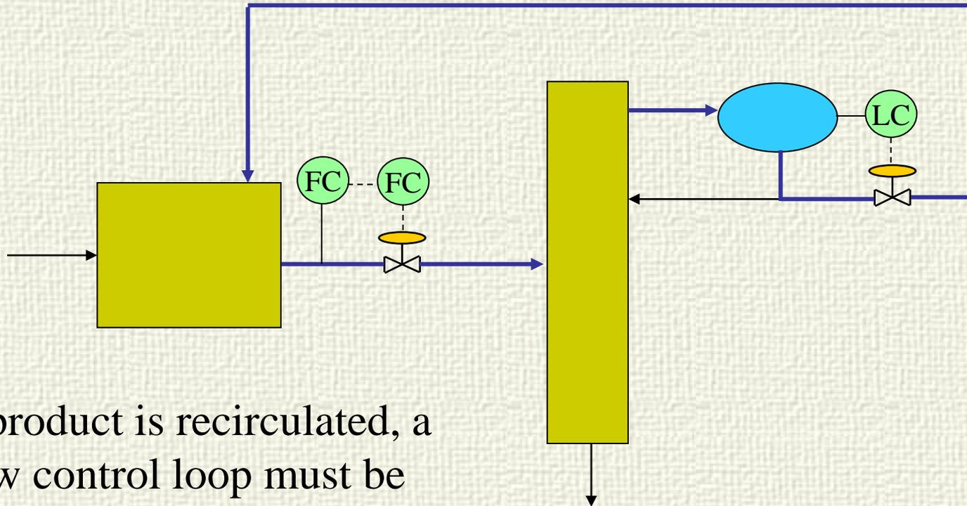
If a product is recirculated, a flow control loop must be placed somewhere in the loop
