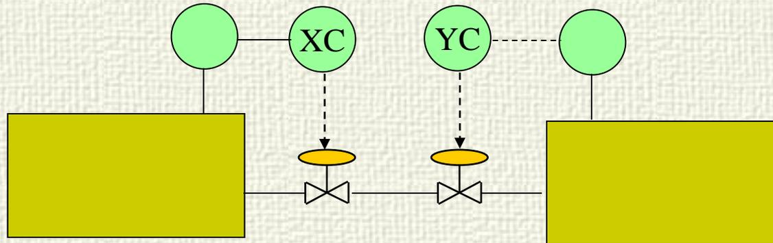
Only one automatic valve is allowed in a pipe
