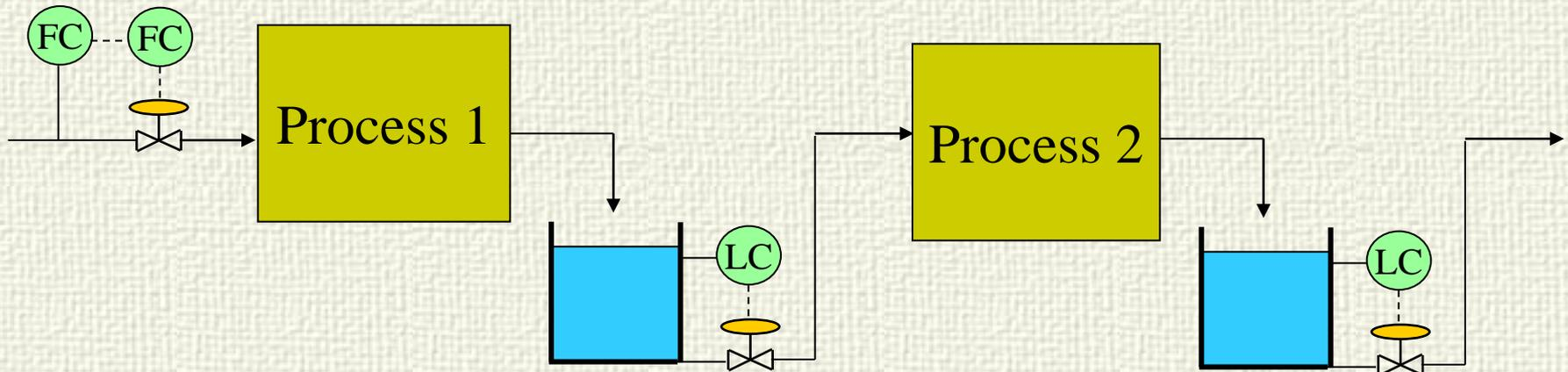
Level control loops must operate in the same direction (backward, forward) according to the point that fix the flow
