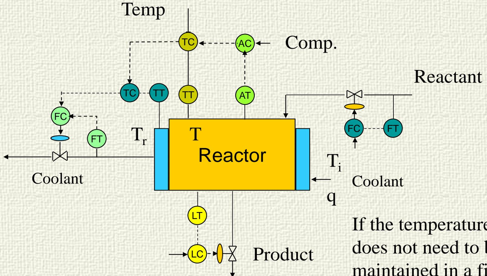
If the temperature does not need to be maintained in a fix value
