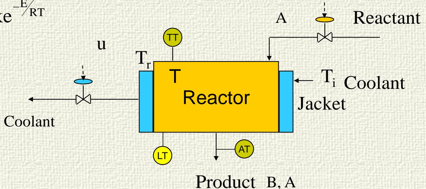
Conversion can be controlled either with the retention time or temperature
