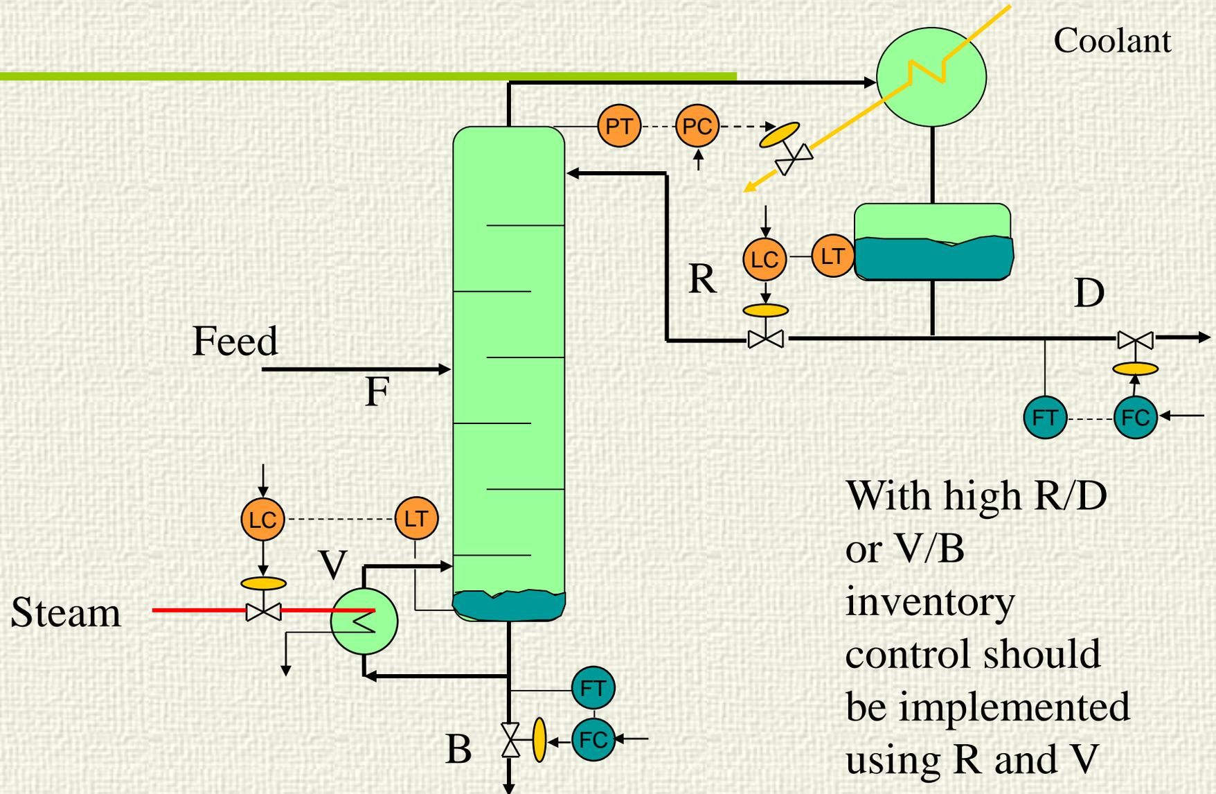
With high R/D or V/B inventory control should be implemented using R and V
