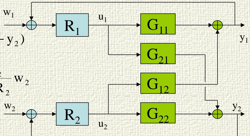
$$y_1 = \frac{G_{11}R_1}{1+G_{11}R_1}w_1 + \frac{G_{12}R_2}{1+G_{11}R_1}(w_2 - \frac{G_{21}R_1}{1+G_{22}R_2}(w_1 - y_1) - \frac{G_{22}R_2}{1+G_{22}R_2}w_2)$$
