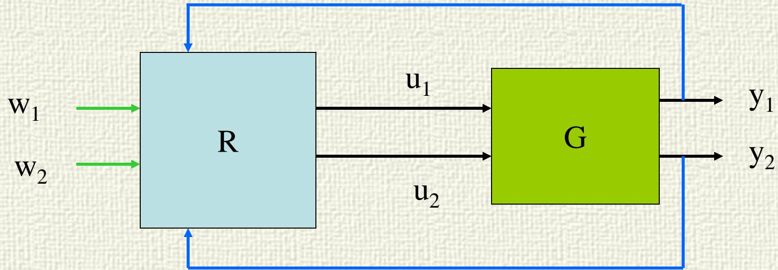
The controller receives signals from all controlled variables (and perhaps measurable disturbances) and computes simultaneously control actions for all actuators taking into account the interactions.
