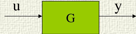
$$G = U\Sigma V^* = \begin{bmatrix} -0.872 & -0.490 \\ -0.490 & 0.872 \end{bmatrix} \begin{bmatrix} 7.343 & 0 \\ 0 & 0.272 \end{bmatrix} \begin{bmatrix} -0.794 & -0.608 \\ 0.608 & -0.794 \end{bmatrix}^*$$
