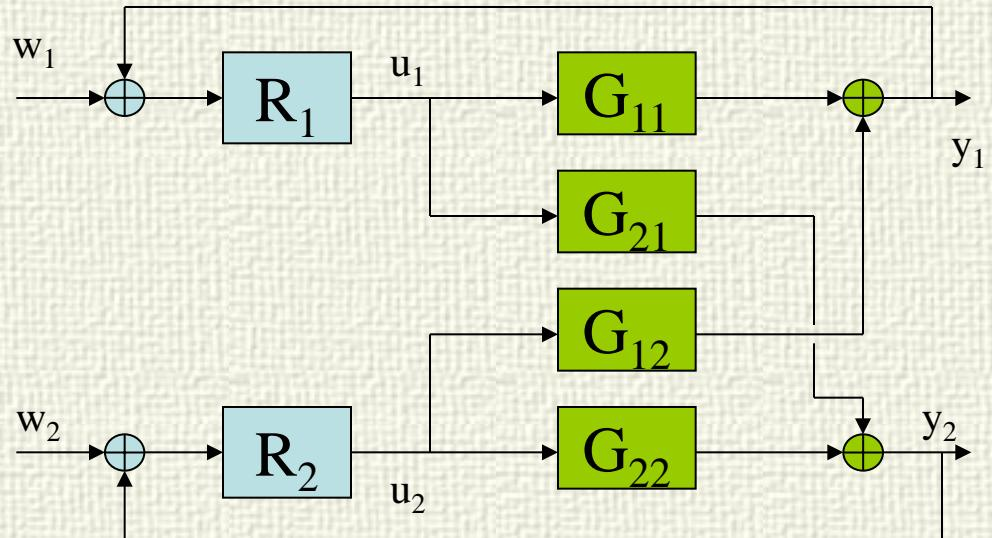
$$y_1 = \frac{G_{11}R_1(1+G_{22}R_2) - G_{12}R_2G_{21}R_1}{(1+G_{11}R_1)(1+G_{22}R_2) - G_{12}R_2G_{21}R_1} w_1 + \frac{G_{12}R_2}{(1+G_{11}R_1)(1+G_{22}R_2) - G_{12}R_2G_{21}R_1} w_2$$
