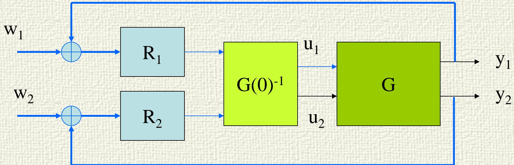
If  $D$  is chosen as  $\alpha G(0)^{-1}$ , then  $G(s)$   $G(0)^{-1}$  is diagonal in steady state, so that there is no interaction at equilibrium. This decoupler is very easy to compute and implement because  $G(0)^{-1} = \text{inverse of the steady state gain matrix}$
