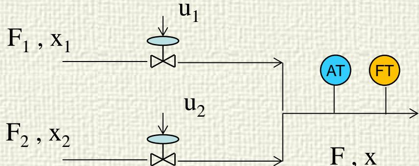
$$x = \frac{F_1 x_1 + F_2 x_2}{F_1 + F_2} \quad \Delta F = \Delta F_1 + \Delta F_2$$
