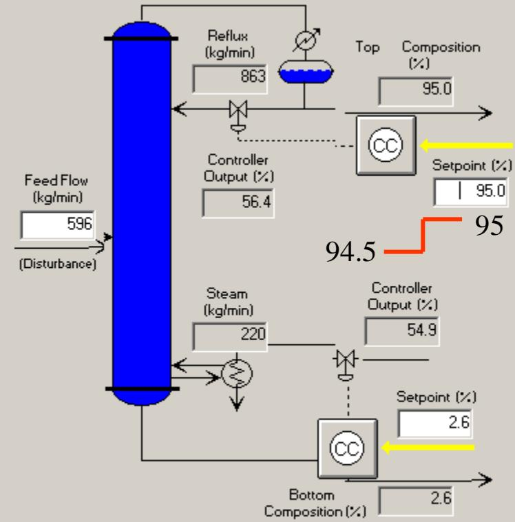
Controllers tuned independently with the other loop in manual
