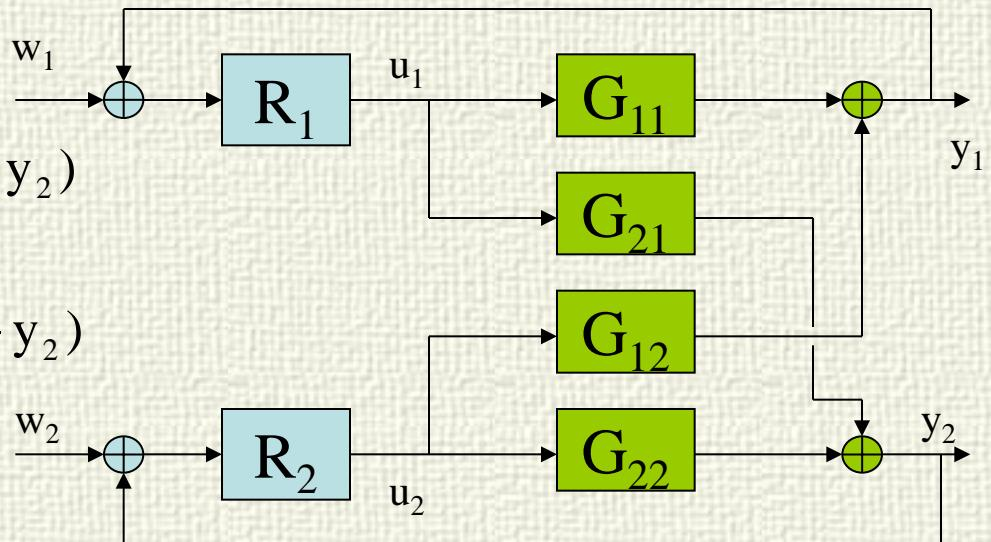
$$y_1 = \frac{G_{11}R_1}{1+G_{11}R_1}w_1 + \frac{G_{12}R_2}{1+G_{11}R_1}(w_2 - y_2)$$
